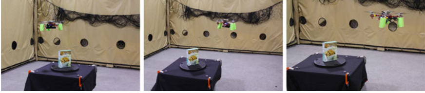
Fig. 4 Quadcopter experiment and test setup. The quadcopter robot, equipped with a RGB-D camera, collects multiple views of a target object (e.g., a cereal box) in an active object recognition task
