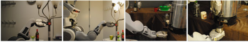
Fig. 8 Examples of transferred trajectories being executed on PR2. On the left , PR2 is able to rotate the ‘knob’ to turn the lamp on. On the right , using two transferred trajectories, PR2 is able to hold the cup below the ‘nozzle’ and press the ‘lever’ of ‘coffee dispenser’
