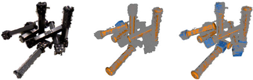
Fig. 2 The illustration of failure cases of ObjRecRANSAC. Figures from the left to right are the testing scene, estimated poses from ObjRecRANSAC and groundtruth
