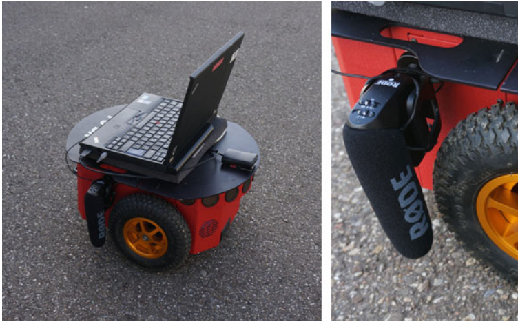
Fig. 2 The Pioneer P3-DX platform showing the shotgun microphone with the shock mount, mounted close to the wheel
