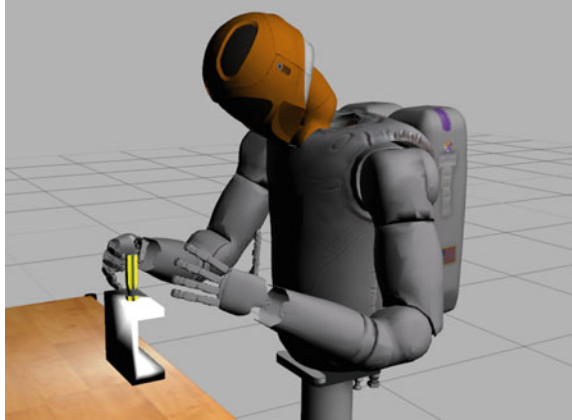
Fig. 5 Robonaut 2 approaching a pregrasp pose for a screwdriver on a tool stand in simulation
