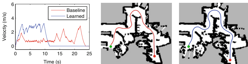
Fig. 6 Experiment in which our planner ( blue ) reached its goal over 2x faster than baseline ( red ). Velocity profiles and trajectories for each planner are shown
