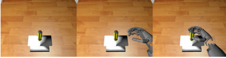
Fig. 6 The first, second, and third aspect stored in the ATG model through demonstration are shown from left to right . In the first aspect, the object on top of the table is a screwdriver on a tool stand. In the second aspect, the robot hand is in a position where a straight movement toward the screwdriver would lead to a pregrasp pose. The third aspect represents a pregrasp pose. This is the goal aspect for the pregrasp task designed in this experiment
