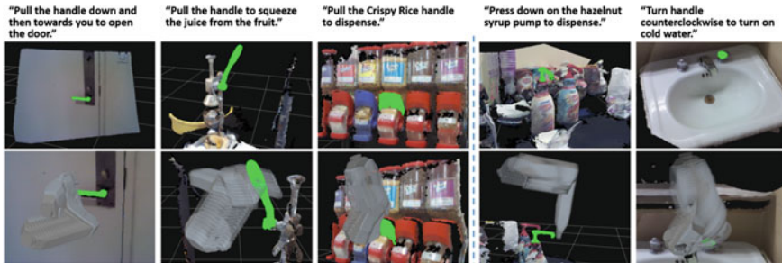
Fig. 5 Examples from our dataset, each of which consists of a natural language instruction ( top ), an object part in point-cloud representation (highlighted), and a manipulation trajectory ( below ) collected via Robobarista. Objects range from kitchen appliances such as stove and rice cooker to urinals and sinks in restrooms. As our trajectories are collected from non-experts, they vary in quality from being likely to complete the manipulation task successfully ( left of dashed line ) to being unlikely to do so successfully ( right of dashed line )
