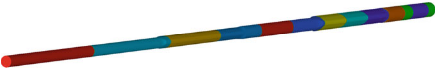
Fig. 18 Bar of the multi-stand Kocks rolling partitioned on 12 processors
