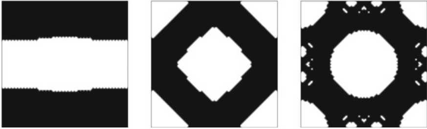
Fig. 2 Horizontal, shear and bulk stress-state optimal RVE topologies
