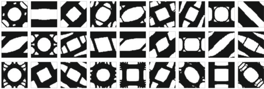
Fig. 11 Typical micro-structure topology outputs of the Computational Vademecum
