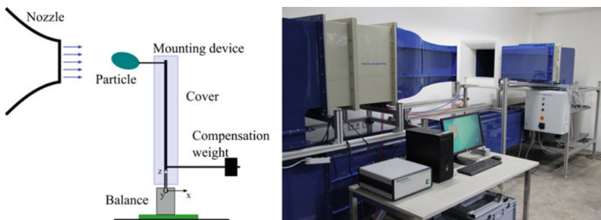
Fig. 3 Schematic of the measurement arrangement (left) and closed wind tunnel test facility (right)
