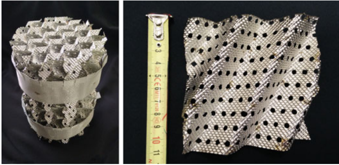
Fig. 1 Example of separation column packing – Mellapak 250X. An overall view of the packing is depicted on the left. On the right, a detail of one element of a dismantled packing is shown. Structured packing usually consists of corrugated, perforated and textured steel plates. The standard mode of operation is counter-current: the liquid phase flows down and the gas phase up
