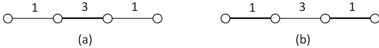
Fig. 1. Matching with maximum weight of edges (a) and matching with maximum cardinality (b)
