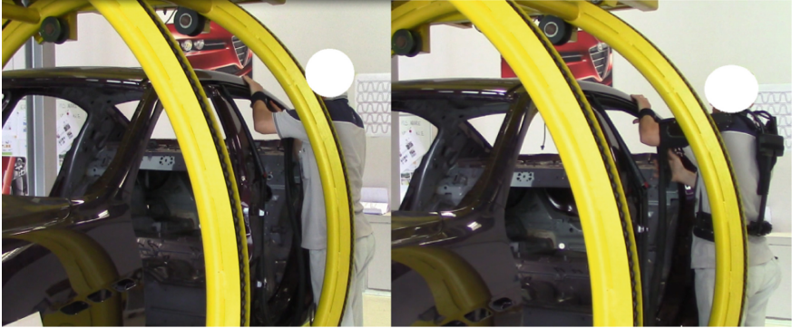
Fig. 4. Mounting the seal on the rear door without and with the exoskeleton
