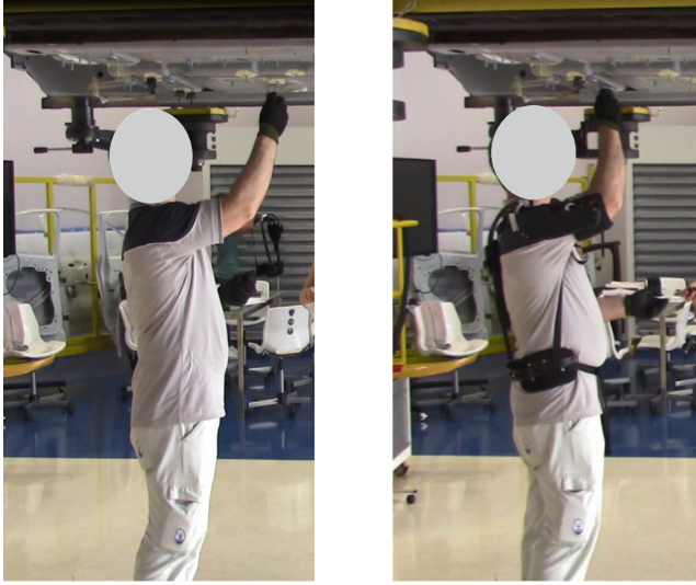
Fig. 2. Mounting the clips of brake hoses underbody without and with exoskeleton
