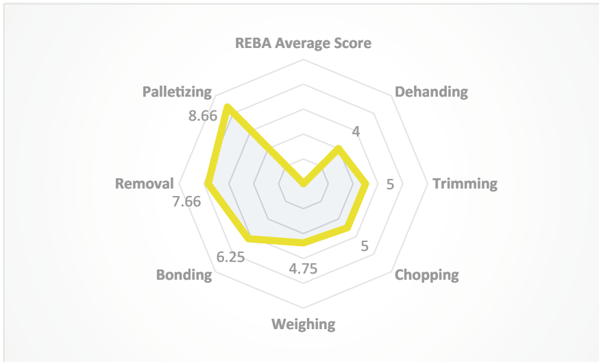
Fig. 1. Final score REBA in each activity of the cultivation and production of banana
