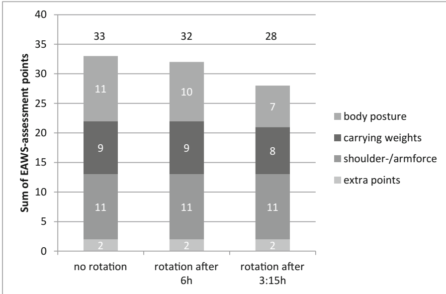
Fig. 1. Workload assessment of assembly activity and sedentary activity for three different job rotation schedules.
