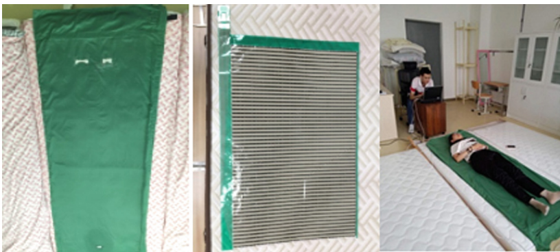
Fig. 2. Mattress pressure sensor for testing and test photo
