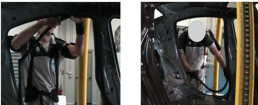
Fig. 5. Potential interference of the exoskeleton with the car frame
