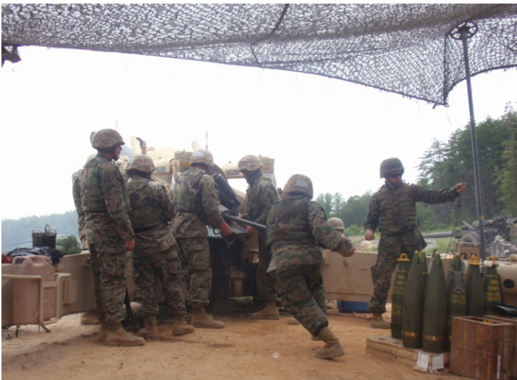
Fig. 2. Two handlers position the tray in front of the barrel as the rammer forces the round into the barrel
