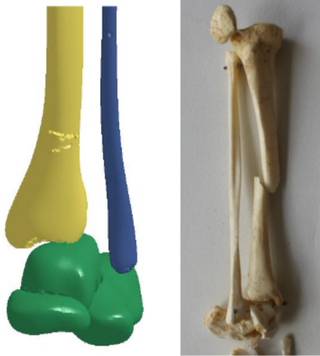
Fig. 5. Numerical and experimental results of frangible leg worn Type-2 boot sample after explosion.
