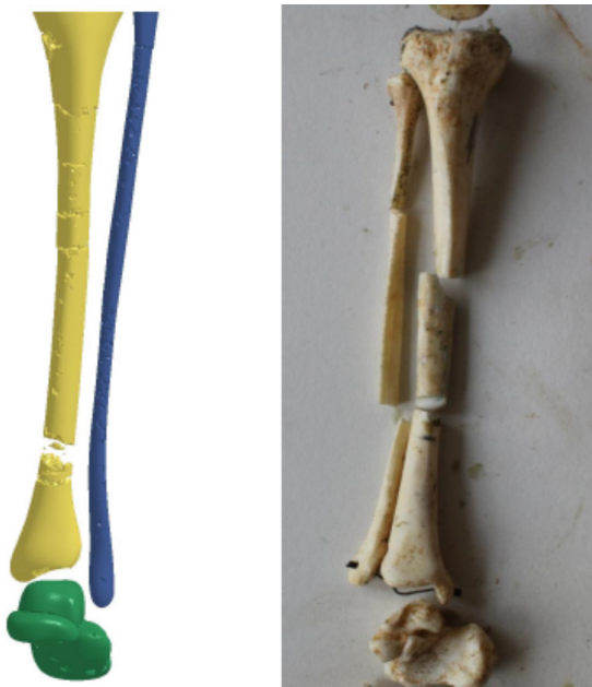
Fig. 2. Numerical and experimental results of frangible leg worn Type-1 boot sample after explosion.
