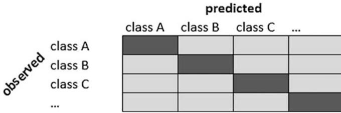
Fig. 3 LUC matrix comparing observed and predicted LUC. Accurate prediction ( hits ) are located on the matrix diagonal ( dark cells ), errors in the rest of the matrix ( light cells )
