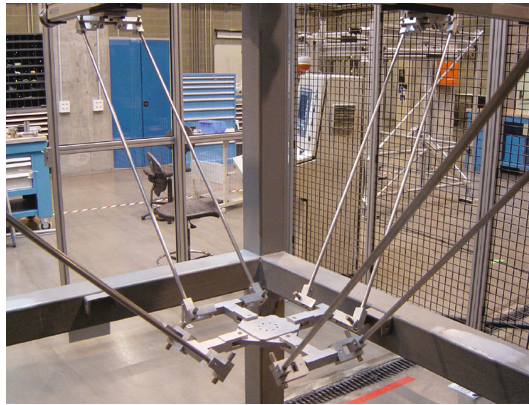
Fig. 1. Prototype of Schönflies parallel manipulator. CompMech research group, department of mechanical engineering UPV/EHU/
