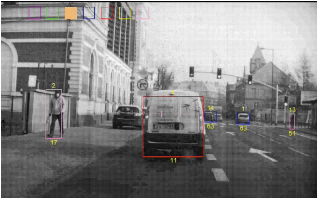
Fig. 2. Data fusion combines radar and camera information for reliable target detection
