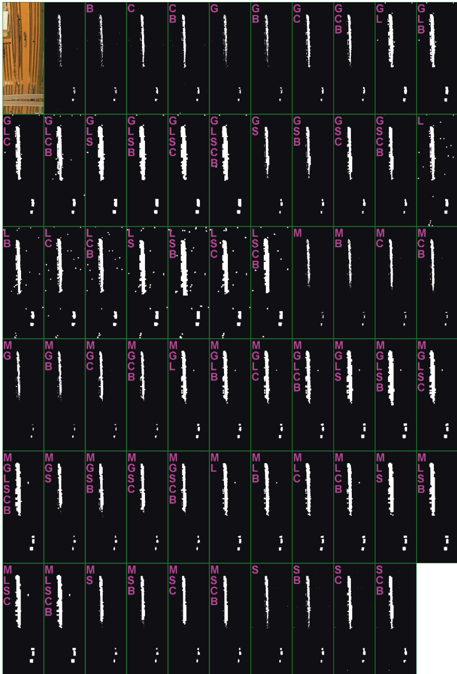
Fig. 9. Original, B&W and 63 combinations of filters ( 5 \times 5 kernel) applied in the following order: G – Gaussian filter, M – median filter, C – morphological closing, L – morphological dilation, S – discretisation (8 px threshold), B – logical sum with previous frame.
