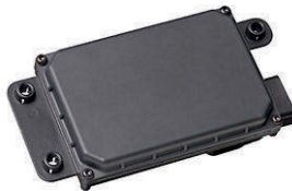
Fig. 1. Example of Medium Range Radar - Delphi MRR.
