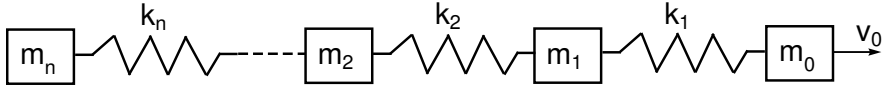
Fig. 4. Mechanical equivalent model of a series of n -cars driving in adaptive cruise control mode
