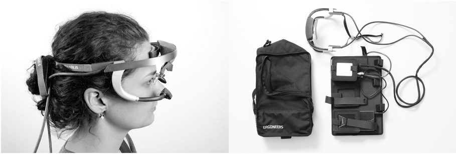
Fig. 1. Head-mounted eye tracking system ( left ) and required equipment for data recording ( right ).
