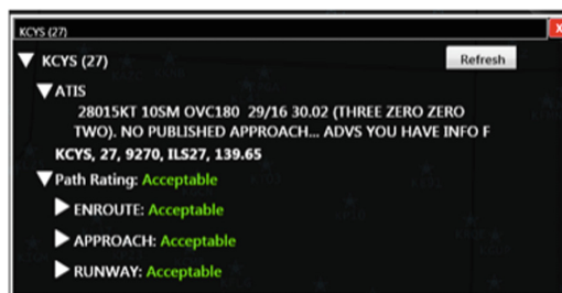
Fig. 4. When using the ACFP, regardless of condition, a transparency window appeared on the TSD for the recommended airport. An ATIS report, runway information, path rating and reasoning statements were also included.
