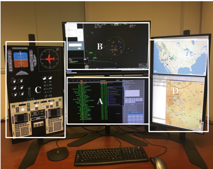
Fig. 1. Simulation ground station. A: Aircraft Control List (ACL), augmented with timeline, alerting information and HAT features. B: Traffic Situation Display (TSD). C: Flight controls and displays for the selected aircraft in read-only mode. D: CONUS map and charts.
