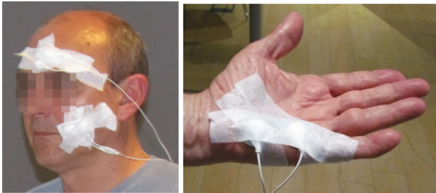
Fig. 1. Facial electromyography ( left ) and galvanic skin response ( right ) electrodes placement.
