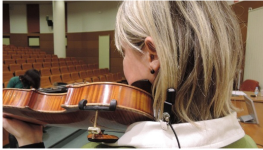
Fig. 4. Location of the Dosimeter microphone during while recording at the hall of the Industrial Engineering School of Leon
