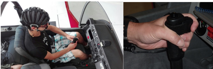
Fig. 1. Left: a participant equipped with the 64-channel Cognionics dry electrodes system. The aircraft was a Robin DR400. Right: the response button attached to the stick.
