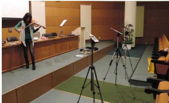
Fig. 3. Location of the Sound Level Meters during the recording at the hall of the Industrial Engineering School of Leon
