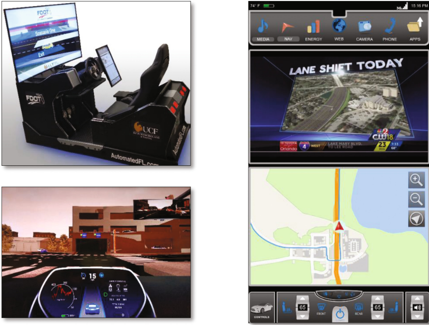
Fig. 2. Final simulation testbed. Top left: A side view of the complete simulator system. Right: The complete interactive dashboard console display showing the routing and media player panes. Bottom-left: A view from the main screen of the simulator as vehicle navigates environment. The dashboard iconography emulates (with permission) that of the Tesla Model S.
