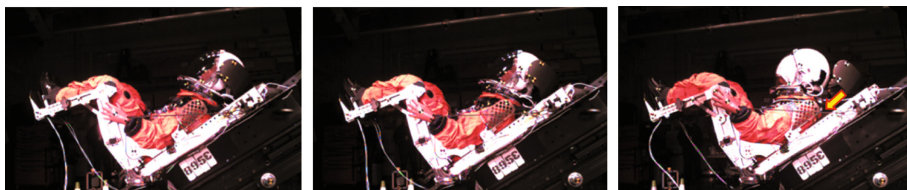
Fig. 2. Motion of the suited small female HIII ATD during HIA testing
