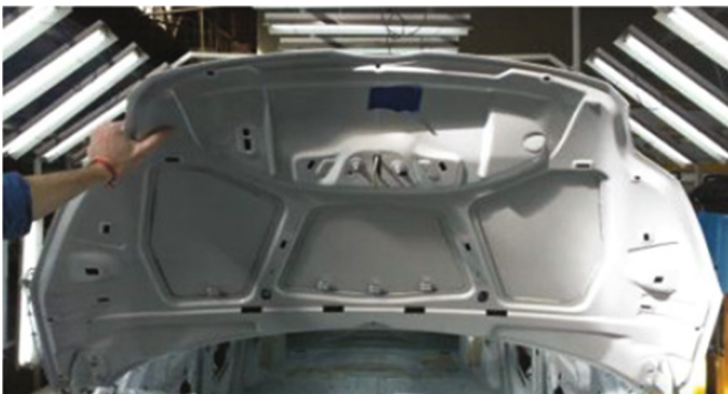
Fig. 4. A marking was made on the hood in blue, in order to be able to place the dynamometer during the movement to open hood.
