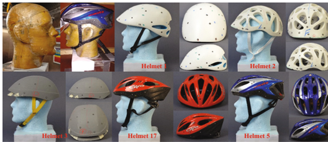
Fig. 1. Nude headform and helmets used for testing in wind tunnel
