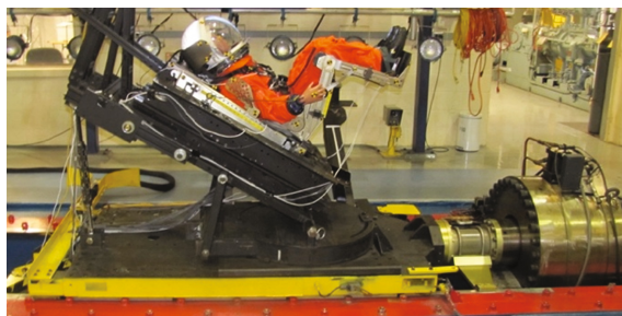
Fig. 1. Suited small female HIII ATD in HIA facility ( hydraulic piston shown on right ).
