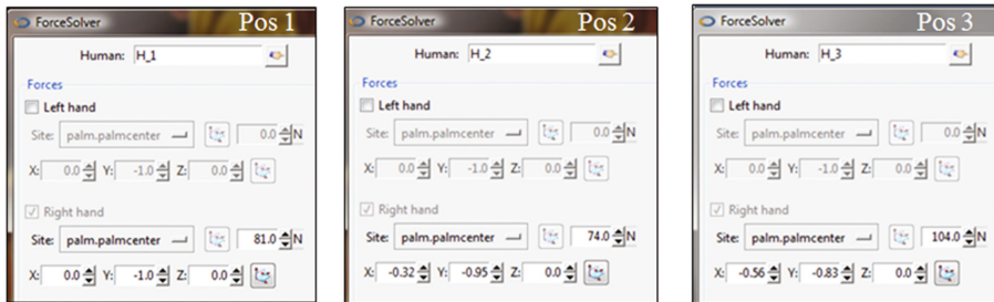
Fig. 9. The Force Solver or strength capabilities for posture 1, posture 2 and posture 3 at same position as CAD and real-life.
