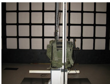
Fig. 5. View of anechoic chamber with radio station during of measurements
