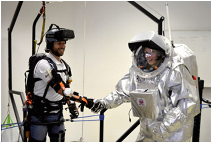
Fig. 5. Motigravity system (left) with elements of the Aouda.X spacesuit (right) to mimic the movement restrictions of the spacesuit ((c) OeWF/Paul Santek).
