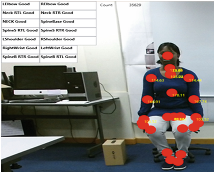
Fig. 2. Neutral position for seated human as specified by the tool
