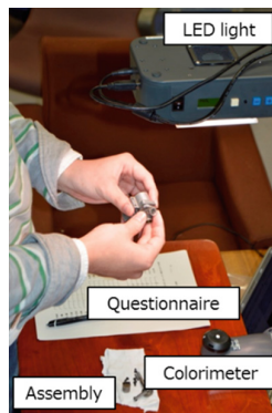
Fig. 1. Circumstance of the preliminary experiment. The LED light illuminates the assembly parts as a task lighting.
