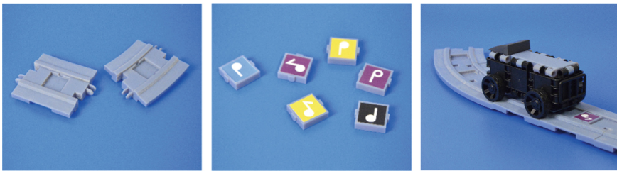
Fig. 1. Prototype of a programmable toy train with a TUI based on tokens. Three different type of game elements. Left non-interactive construction elements. Central tokens. Right electronic reading system.
