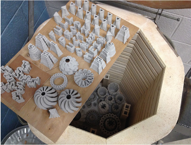
Fig. 3. 3D printed ceramic type and objects
