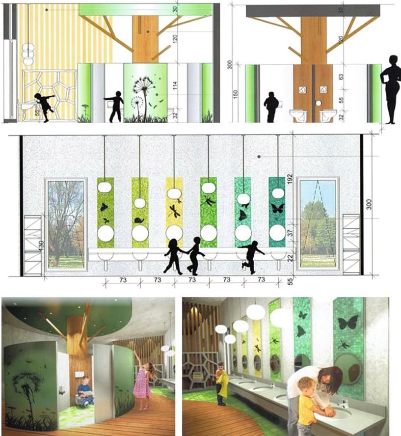
Fig. 2. The Meadow - example of shaping the kindergarten bathroom, wall elevation views and perspective views (Source: student project depicted by K. Kepka, tutor - A. Jaglarz)
