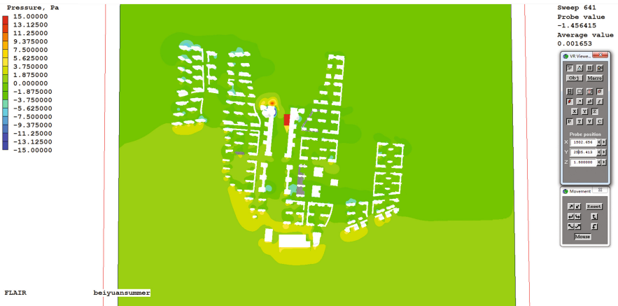
Fig. 9. Jinan Riverfront District North lake area conceptual design. Line height wind pressure distribution in summer.
