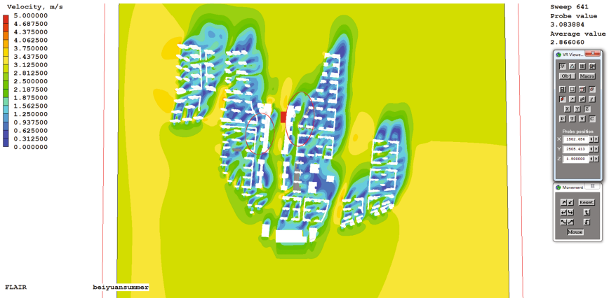
Fig. 8. Jinan Riverfront District North lake area conceptual design. Line height wind pressure distribution in summer
