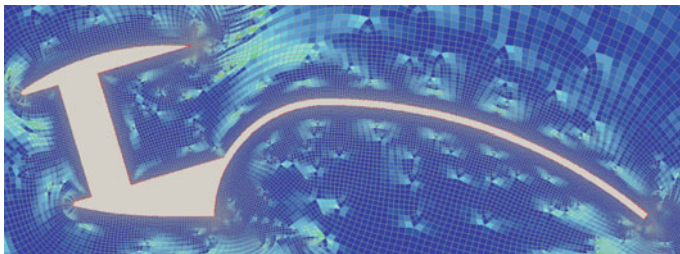
Fig. 9 Skewness analysis of the mesh around a wing profile (max visible skewness 1.5 green cells in the visualized area)
