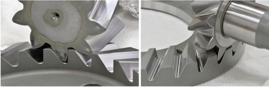
Fig. 24 IPB gears in good mesh and smooth working
