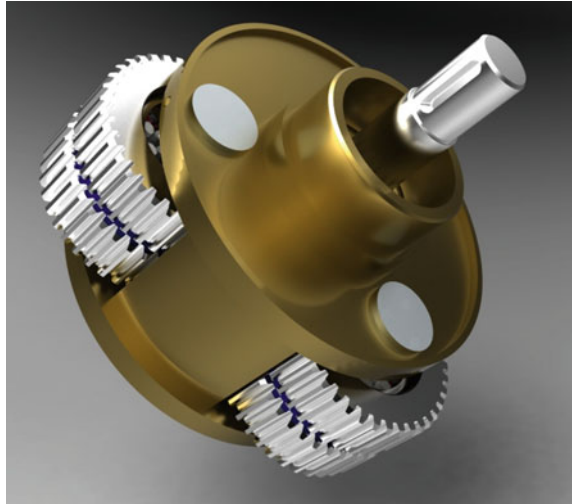
Fig. 20 Assembly unit of satellites for a planetary gear with double-row satellites
