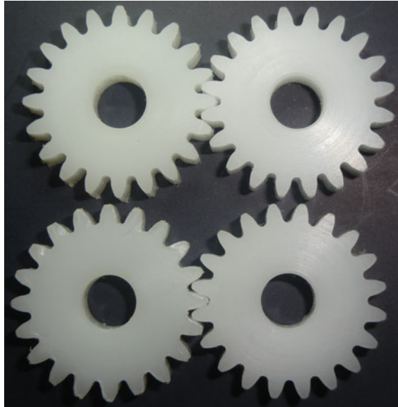
Fig. 7 Involute ( above ) and S-gears ( below ) made of PA66 ( left ) and POM-C ( right )
