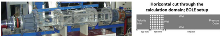
Fig. 4 EOLE test section with an 8 row rod bundle in place (30° slope angle); calculation domain
