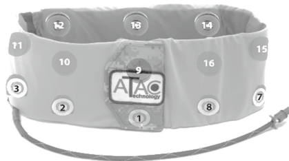
Fig. 1. Dual Belt (Engineering Acoustics, Inc.) tactile display comprising of a row (1–8) of eight EMR motor based tactors and a row (9–16) of eight C-3 tactors. The Dual Belt is constructed using stretchable material, with each tactor in a pod. The belt closure in the front using an overlap to accommodate the belly tactor (1 and 9) and electronic connection through an egress connector.
