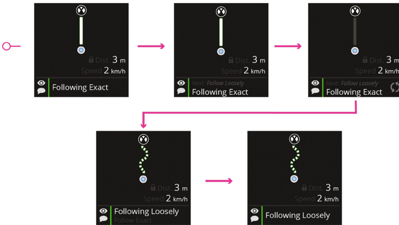
Fig. 3. A series of screens illustrating the Command Status Region, which appears below the Tracker View and provides observability of command status, including receipt of the command, processing, and acceptance/execution. This display region uses variable salience and integrates with the Tracker View to promote operator understanding of command status.
