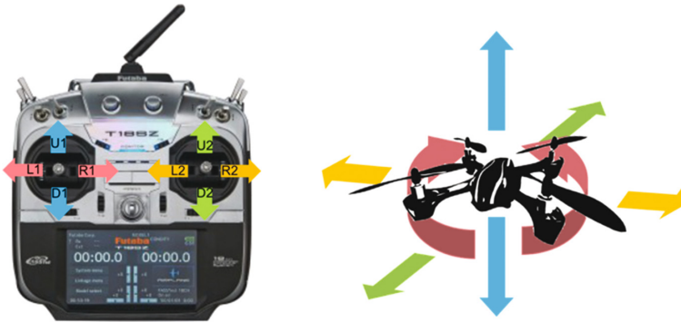
Fig. 1. Typical legacy controller and movement designations for sUAS control.
