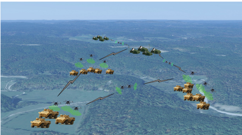
Fig. 4. A concept of drone relay stations (DRS)
