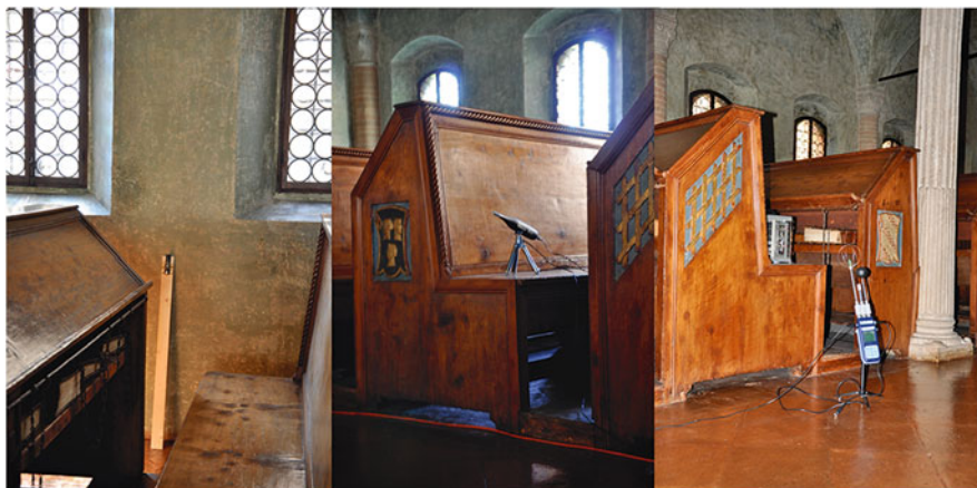
Fig. 4.2 Positioning of probes in Malatestiana Library from the left to the right: air temperature probe; CO 2 sensors; microclimate datalogger
