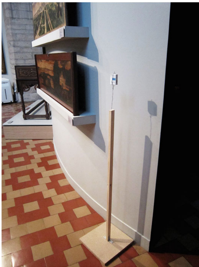
Fig. 11.4 Hobo U12 data logger during the installation on dedicated support
