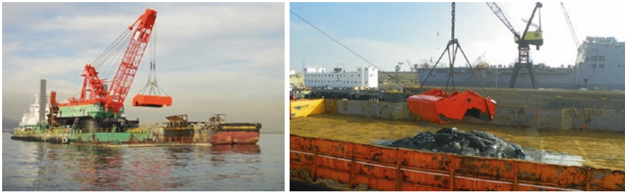
Fig. 10.3 Mechanical Dredges: Environmental Closed Buckets Courtesy of Cable Arm Company
