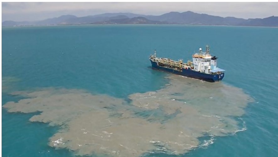
Fig. 10.15 A hopper dredge disposing dredged material. Courtesy of Cairns Post
