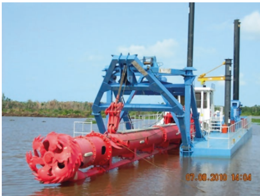
Fig. 10.4 Typical hydraulic cutterhead dredge. Courtesy of Ellicott Dredges Company
