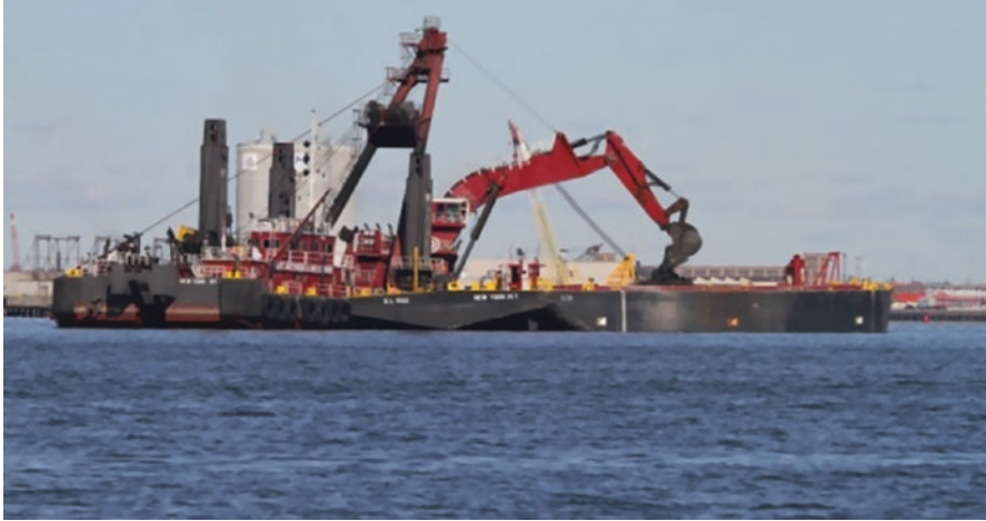
Fig. 10.2 Mechanical backhoe with articulated arm on dredge New York . Courtesy of Great Lakes Dredge & Dock Company
