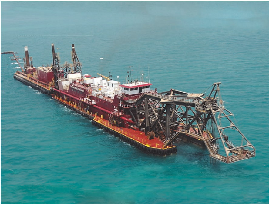
Fig. 10.6 Cutterhead pipeline dredge CSD Texas. Courtesy of Great Lakes Dredge & Dock
