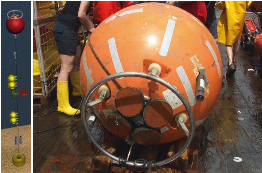
Fig. 1.17 Left: Sketch of a mooring by Mario Müller. An ADCP is mounted into the top buoy of the mooring, a temperature and salinity recorder, yellow floating buoys, a current meter with a large red fin and a pair of grey releasers are attached to the wire between the top buoy and the anchor at the seafloor. Right: Picture of an ADCP mounted within a top buoy after recovery. The four transducers send and receive the sound pulses (photo: Tim Fischer)
