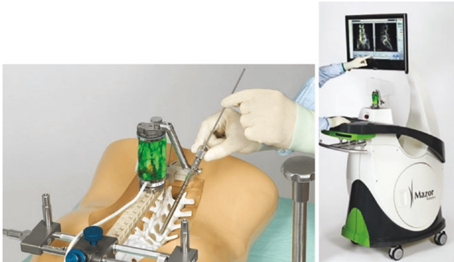
Fig. 3.1 The Renaissance® guidance system, Mazor. With permission from Mazor Robotics, Inc.
