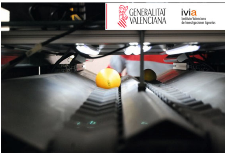
Fig. 4 Machine for the automatic inspection of fruit in-line using computer vision
