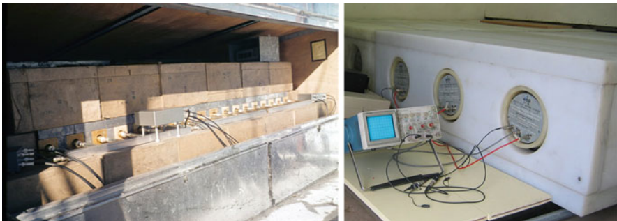
Fig. 6.1 18-IGY neutron monitor Jungfrauoch, Switzerland, ( left ) and 6-NM64 neutron monitor Athens, Greece ( right ). The digits 18 respectively 6 give the number of the counter tubes of the corresponding neutron monitor station
