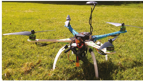
Fig. 1. One of the quad-copters considered (named as “Q1”). Each model requires one li-po battery which perform until 15 min of flight. However, to preserve life of the battery, each flight with the cameras was performed in less than 6 min.
