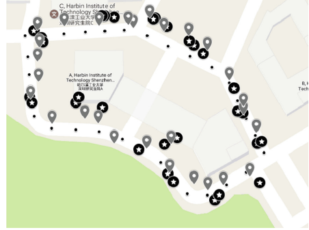
Fig. 6. Distribution of pre-calibrated points, GPS positioning results and Our hybrid results, represented by black dots, gray icons and black star icons respectively.
