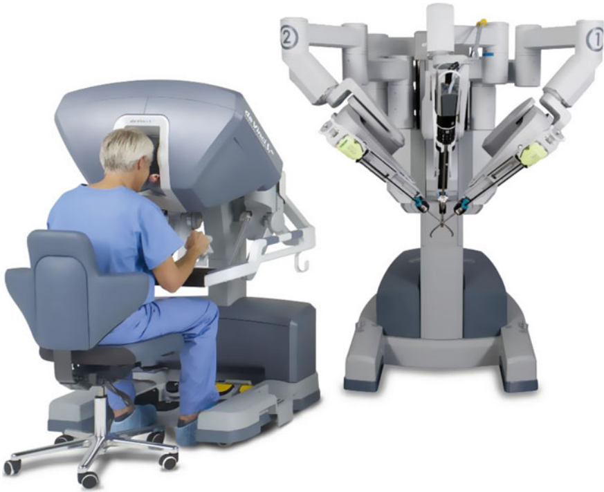
Fig. 2 Da Vinci Si system with Single-Site™ instruments. © 2009 Intuitive Surgical, Inc
