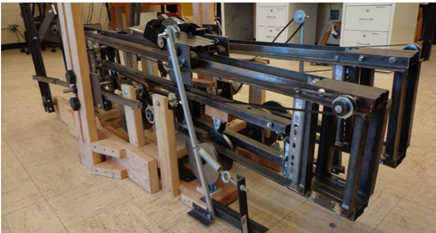
Fig. 1 Initial prototype of gait rehabilitation robot (as in [8])
