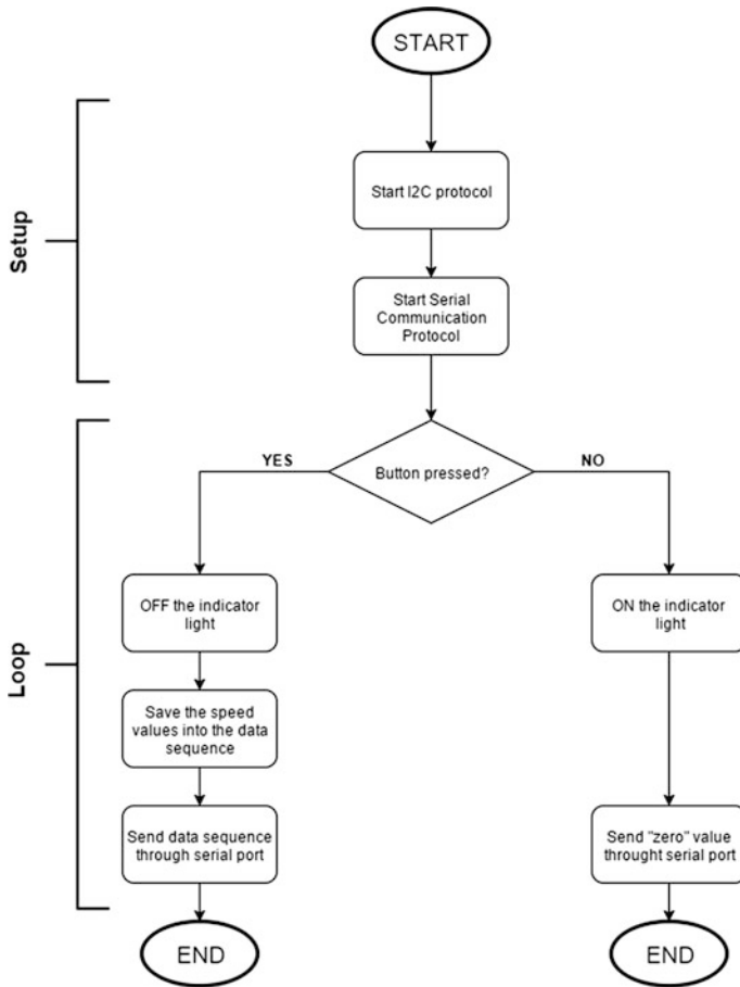
Fig. 7 The flowchart of the program on Arduino board
