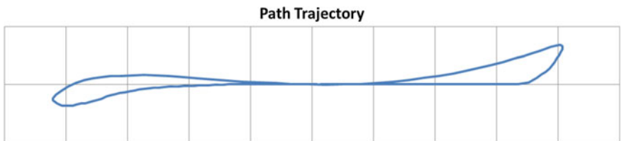
Fig. 6 Crank-slider compatible path trajectory
