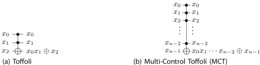
Fig. 1. Basic reversible gates
