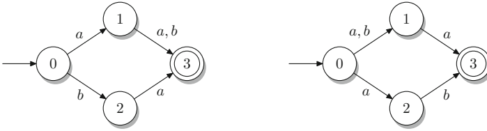
Fig. 1. A minimal NFA (left) and a minimal REV-NFA (right) for the finite language L = \{aa, ab, ba\} . Thus, L is a nondeterministically reversible language.
