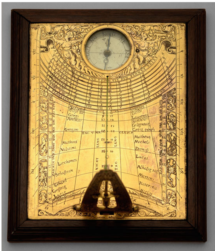
Fig. 8.17 A work planner. String-gnomon dial by Ulrich Schniep, Munich, 1572, showing the hours of daylight available each month. Adler Planetarium, Chicago, M-243
