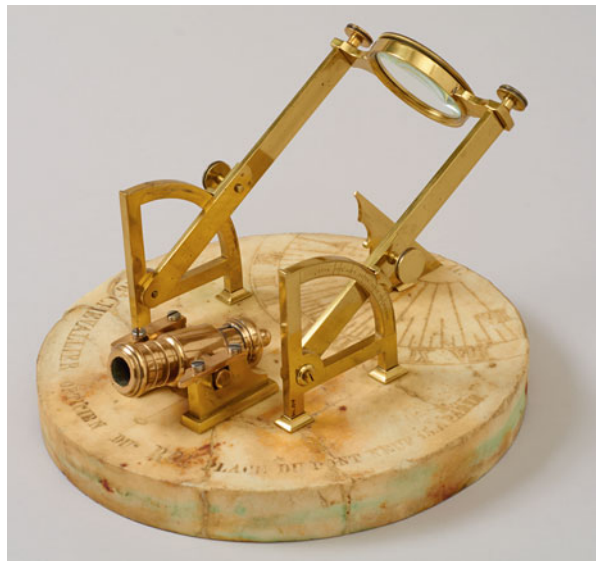
Fig. 8.24 An acoustic sundial to regulate clocks. Cannon dial by Jean-Gabriel-Augustin Chevallier, Paris, circa 1820. Adler Planetarium, Chicago, W-104
