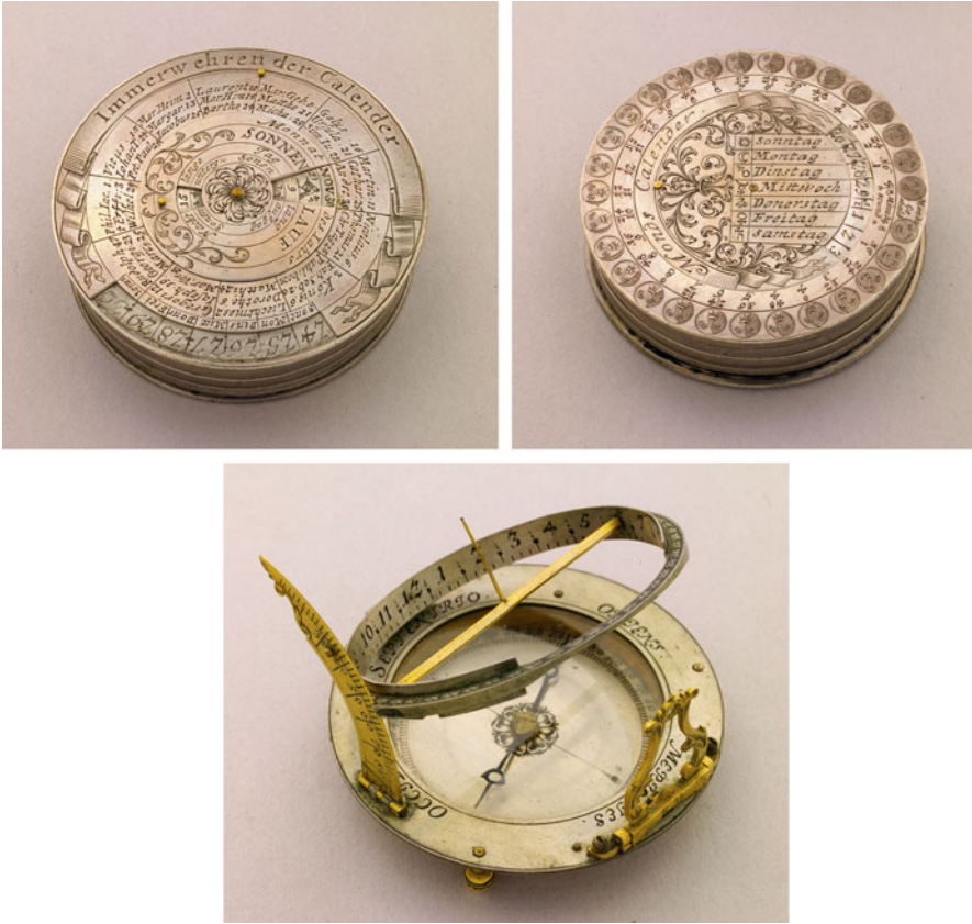
Fig. 8.5 A perpetual calendar to keep track of religious festivals and lunar phases, engraved on the silver case of an Augsburg-type dial by Johann Martin, Augsburg, 1671–1719. Adler Planetarium, Chicago, A-98
