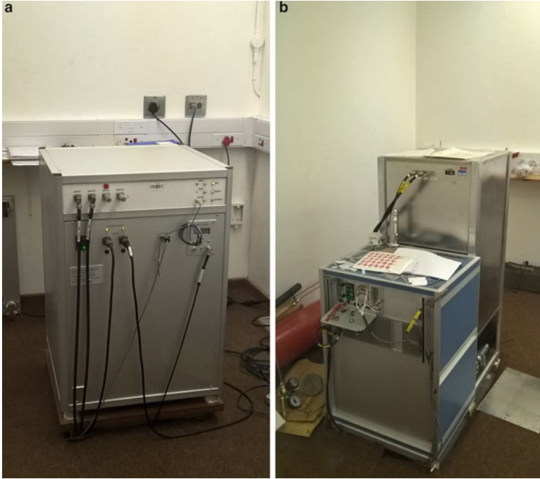
Fig. 29.3 Hydrogen masers at HartRAO; these are located in a thermally stabilized room to reduce thermal fluctuations. (a) Model EFOS-28, installed November 2003, which is an EFOS-C model. (b) HartRAO's first maser (EFOS-6) acquired for VLBI purposes; installed May 1985, this is an EFOS-A model. Not shown is iMaser-72, installed April 2012, which is an iMaser 3000 model. Room temperature is controlled to within \pm 2 °C
