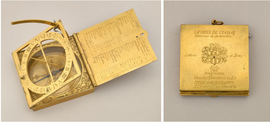
Fig. 8.3 A diplomat's sundial with a secret code. Universal equatorial dial by J. J. Schört, Paris, 1638, owned by Jacques de Stavay, lord of Molondin, Switzerland. Views of the pocket dial with a detail of the underside of the compass box, showing the cipher. Adler Planetarium, Chicago, M-294
