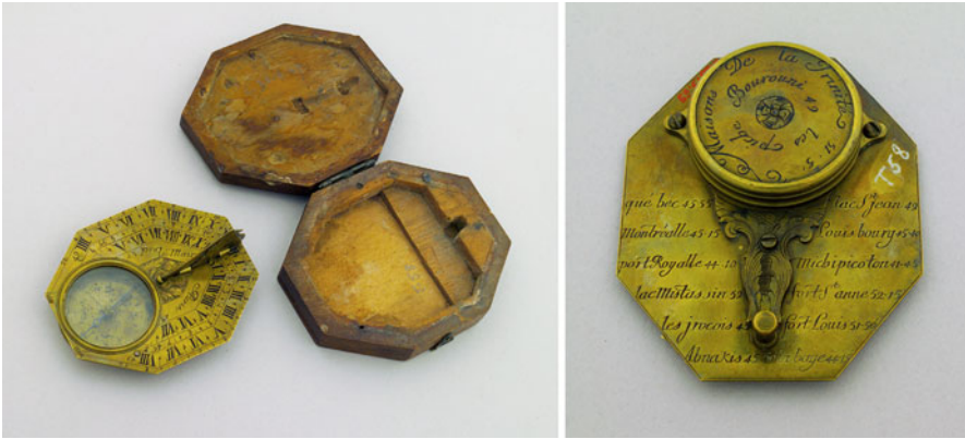
Fig. 8.21 A colonial administrator. Butterfield-type sundial made in Paris by Pierre le Maire II, 1730–1760, for use in New France. The gazetteer lists fur trading posts, forts, and Native American tribes across Canada. Adler Planetarium, Chicago, T-58
