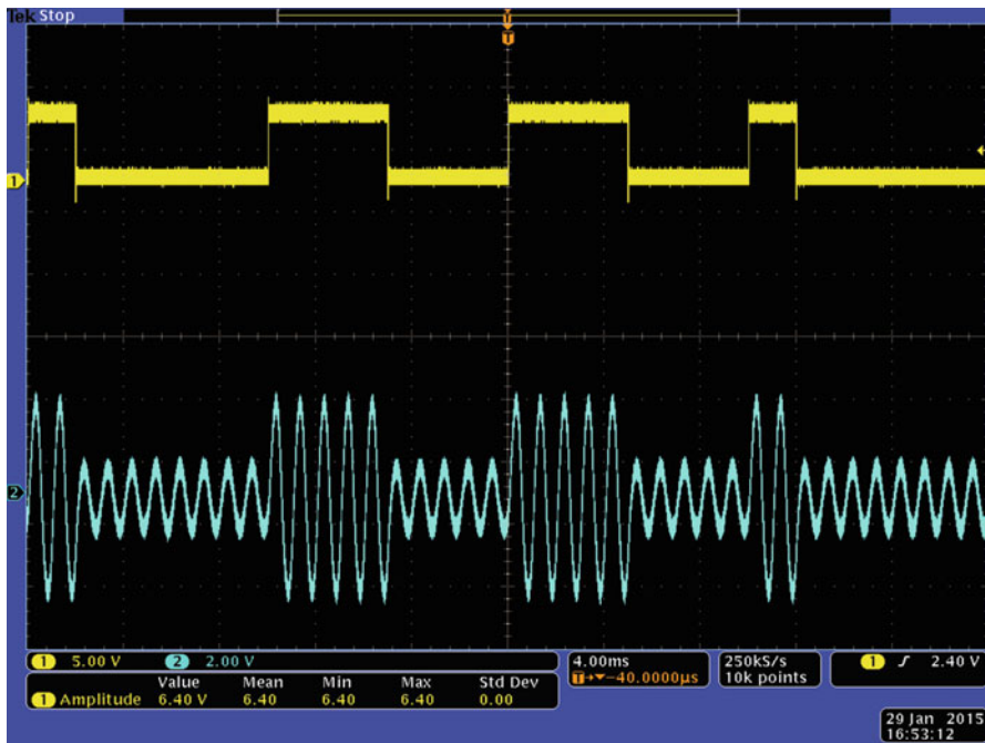
Fig. 38.10 Unmodulated and modulated time code signals
