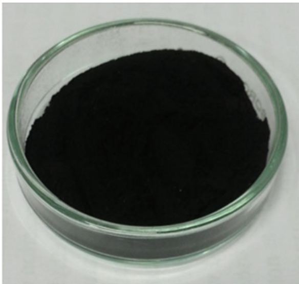
Fig. 5.6 CZTS micropowder after heating at 473 K in air
