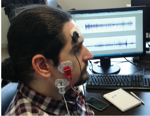
Fig. 2. Recording the myoelectric surface signal produced by the contraction of the masseter.
