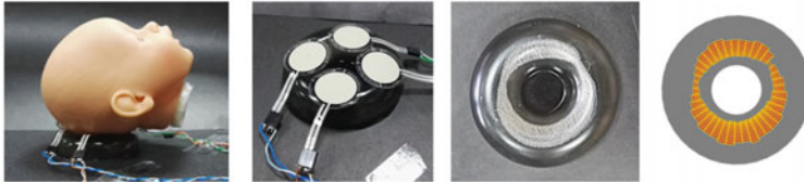
Fig. 1 The three-dimensional anatomical model of the skull, fat and skin tissues and the modeled intrusive medical devices that were tested ( top ). Validation of the modeling using a phantom of a baby’s head on a jelly doughnut embedded with force sensors ( bottom )
