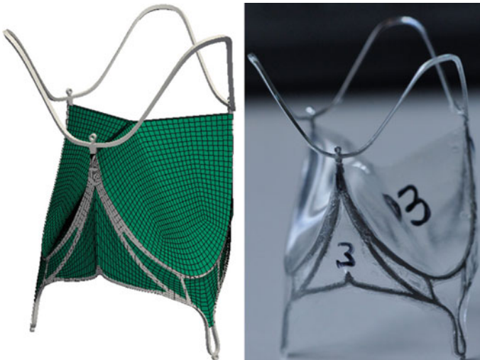
Fig. 1 Nitinol TAV ( right ) and corresponding finite element model ( left )
