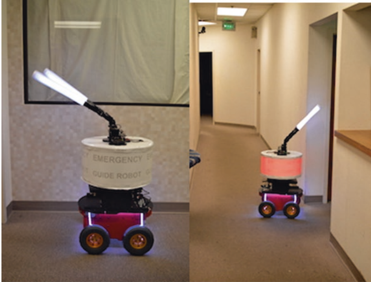
Fig. 6.16 Robot during non-emergency phase of the experiment pointing to meeting room door ( left ) and robot during emergency pointing to back exit ( right ). Note that the sign is lit in the right picture. A standard emergency exit sign is visible behind the robot in the emergency
