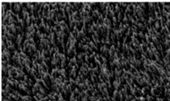
Fig. 12.4 SEM image for Au nanowires, synthesized using AAO membranes
