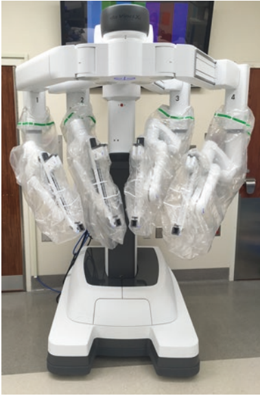
Fig. 5.5 Da Vinci Xi with four robotic arms that are mounted on a mobile overhead boom
