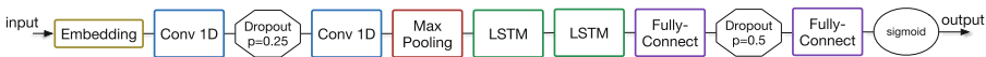
Fig. 12. Network architecture. We use an 8 layer deep learning model. It is primarily built around the LSTM layers, which develop the temporal relationships between instructions. The CNN layers vastly increase the stability of the model while also aiding in preventing it from overfitting. The DNN layers at the end bring everything from the previous layers together in a classification value stating if it was given matching function representations
