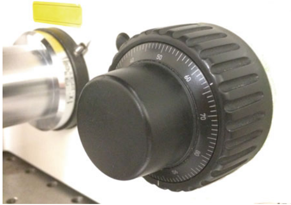
Fig. 3.13 Knob of the microscope used for the adjustment of the focussed image
