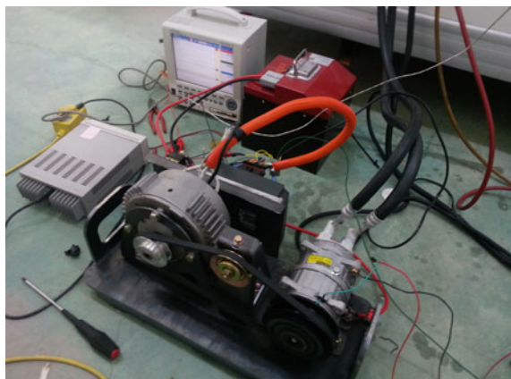
Fig. 4 Test jig for measuring rotating speed and electric power consumption
