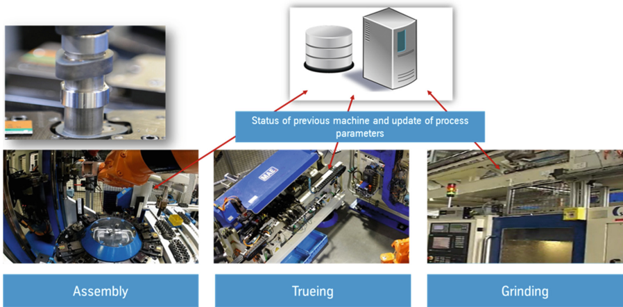
Picture 4. Camshaft production in Ilsenburg
