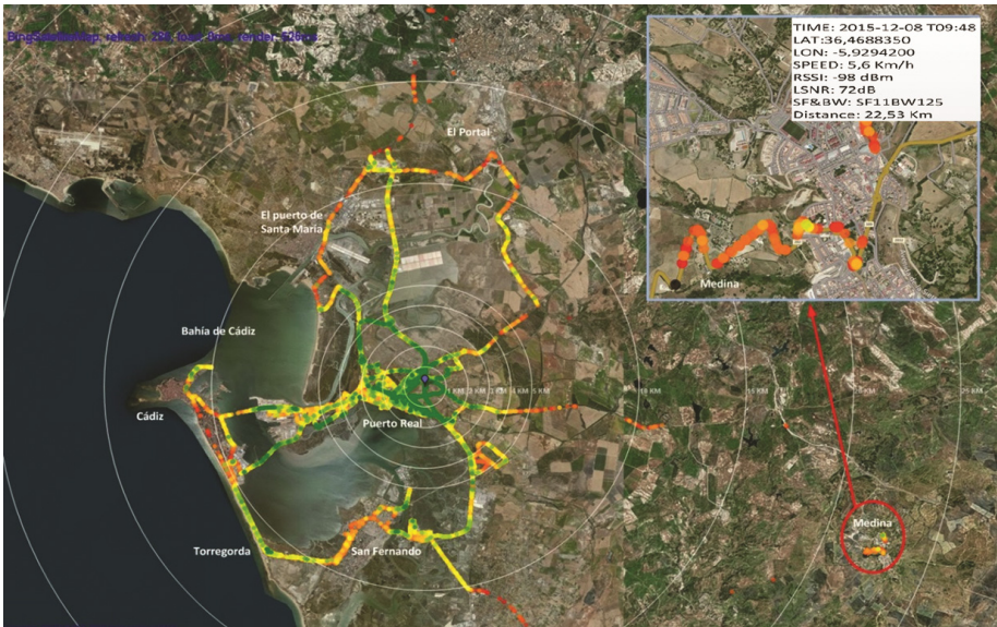
Fig. 6. Map of real coverage obtained as result of test in urban and rural areas around Cádiz
