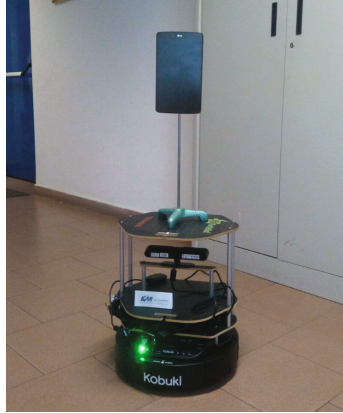
Fig. 8. Turtlebot2 equipped with data logging tablet
