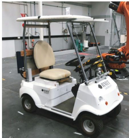
Fig. 3. UGV with control system designed by RMIT (SoE) students of Mechatronics
