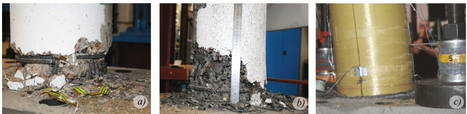
Fig. 5. Failure modes: (a) conventional reinforced concrete D250-R00-F0, (b) rubberised member D250-R60-F0 (c) Confined rubberised member D250-R60-F3
