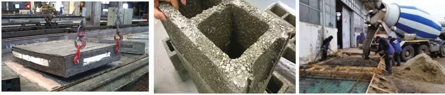
Fig. 2. SUS-CON pre-fabricated components (panels, building blocks) and ready-mixed concrete.
