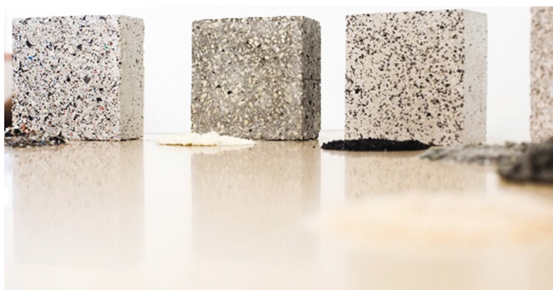
Fig. 1. SUS-CON concrete specimens made of 100% SRM.
