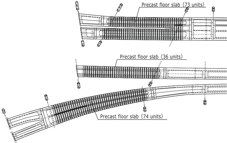
Fig. 10. Plan view of precast floor slabs
