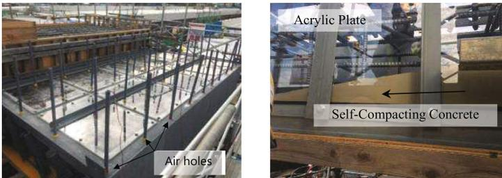
**Photo 1.** Full-scale specimens of joint section (upper flange)
