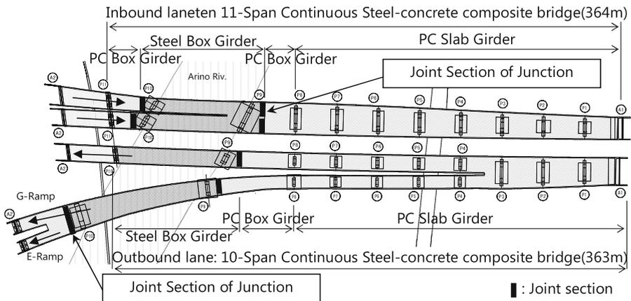
Fig. 2. Plan view of the Arinogawa Bridge
