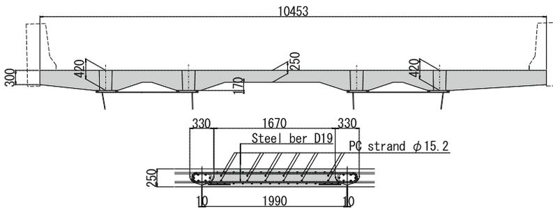
Fig. 11. Section view of precast floor slab (Outbound lane)
