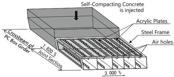
**Fig. 9.** Full-scale specimen of the joint section (upper flange)
