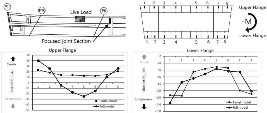
Fig. 7. Axial force of PBL on F-ramp P9 joint section
