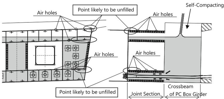
Fig. 8. Point likely to be unfilled of steel cell
