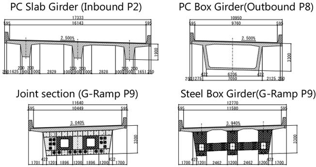
Fig. 3. Cross sectional view of the Arinogawa Bridge
