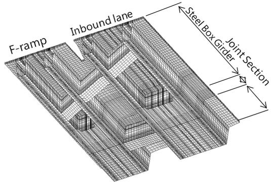
**Fig. 5.** Partial model of FEM analysis (View from below)
