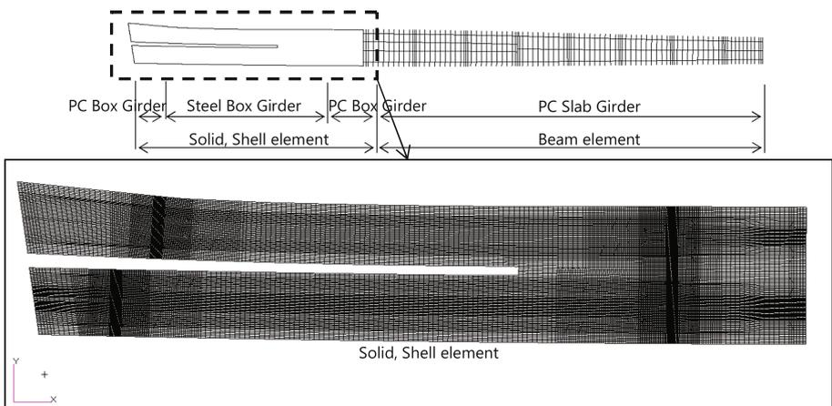
**Fig. 6.** Full-bridge model of FEM analysis
