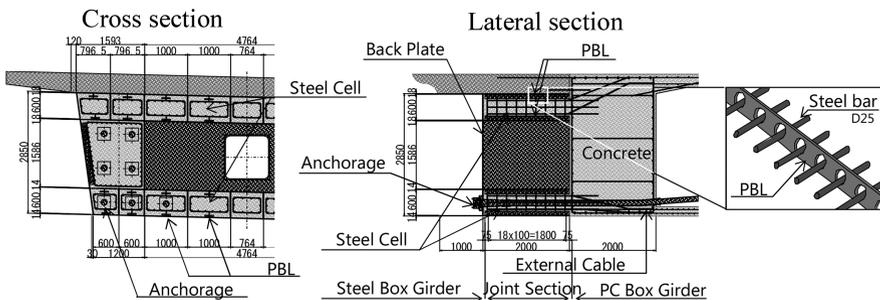
Fig. 4. Structure of joint section
