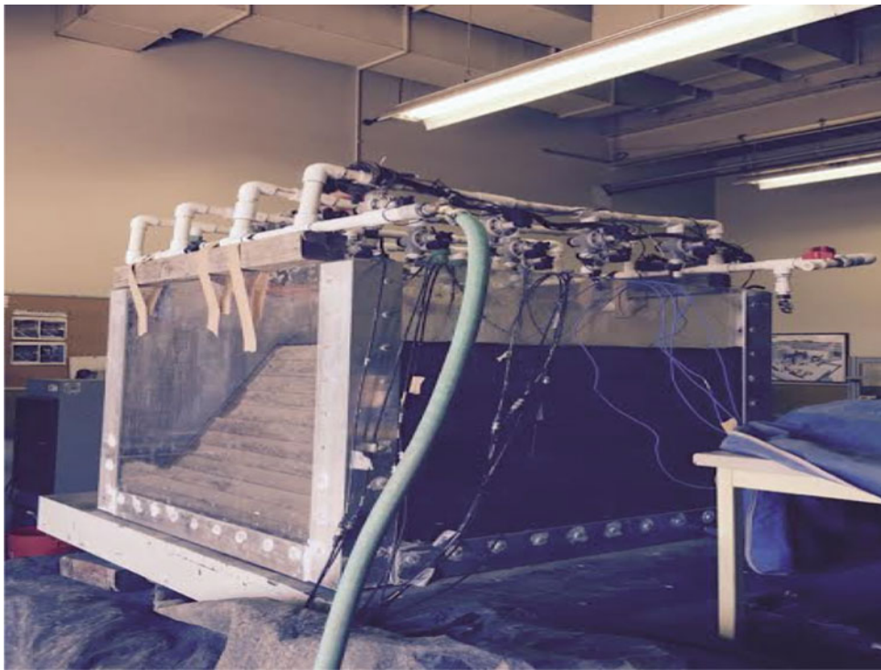
Fig. 5 Rain simulator system on slope model
