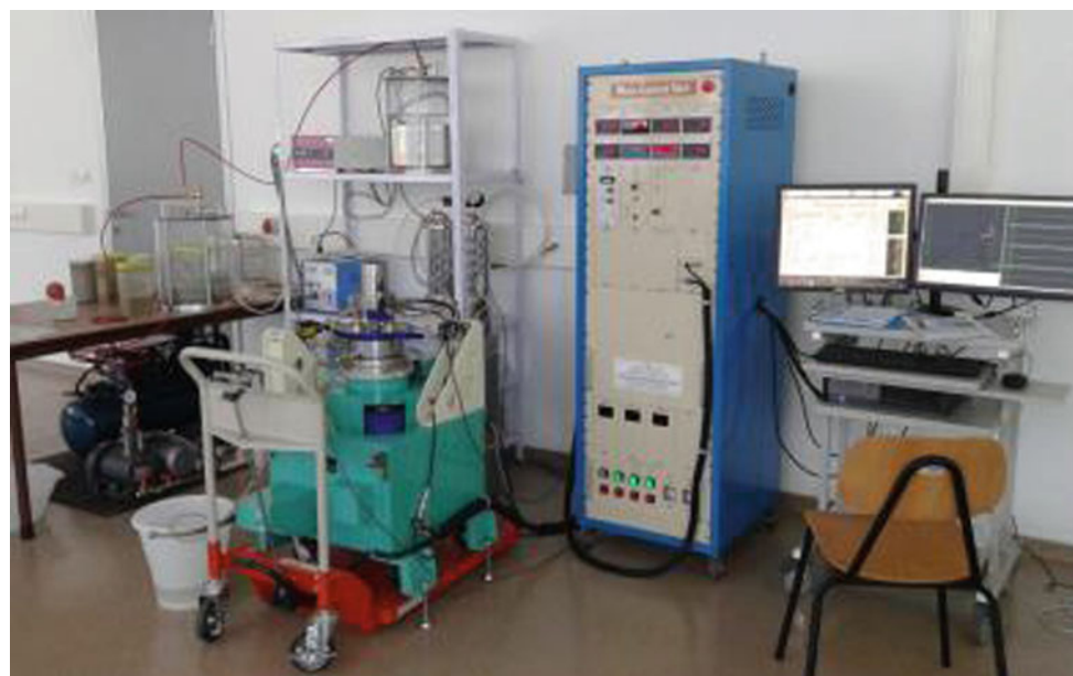
Fig. 10 New developed portable ring-shear apparatus designed for testing under static and dynamic conditions for deep-seated large landslides in Croatia
