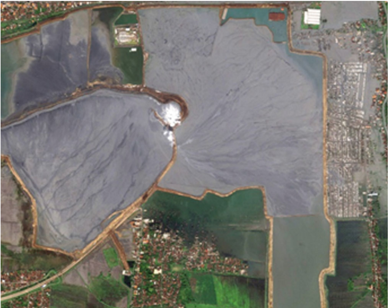
Fig. 4 The spreading of the mud eruption in the district of Sidoarjo and the cells with protection dykes (CRISP)
