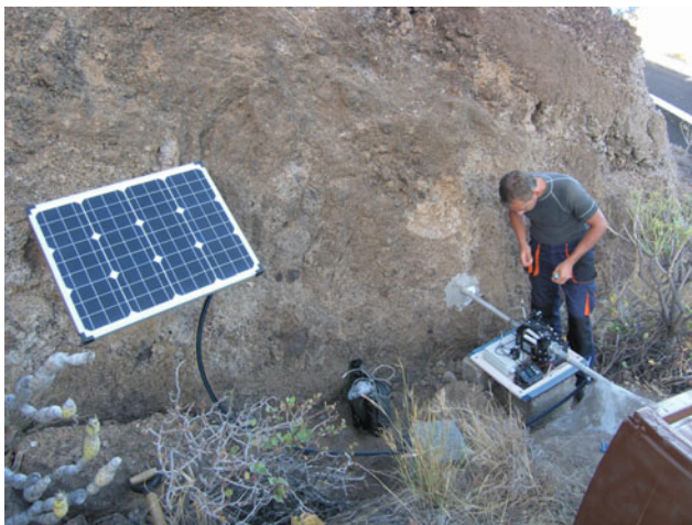
Fig. 1 One of the monitoring sites on the El Hierro Island, Canary Archipelago, Spain. The automatic crack gauge (in front of the person) records movements along a side scarp of the San Andrés deep-seated landslide
