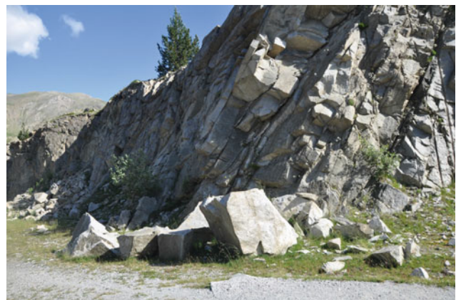
Fig. 10 Rock fall fragmentation by the disaggregation of the original rock mass in Estany Gento, Central Pyrenees, Spain. Most of the block faces are joint planes present in the in situ rock mass. Notice that crushing of the fragments is virtually absent
