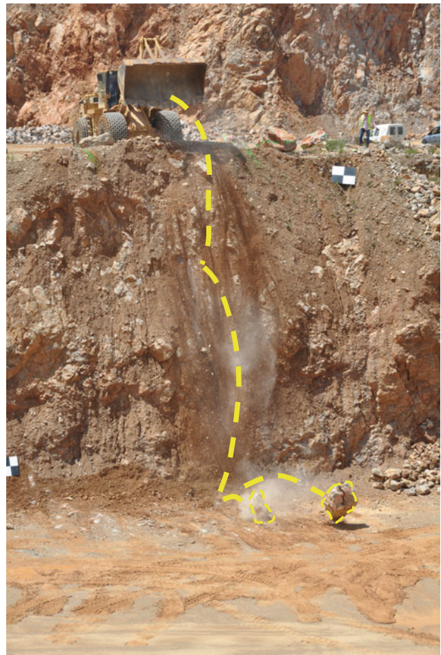
Fig. 9 Block fragmentation by breakage in a real scale test in Vallirana (Barcelona, Spain)
