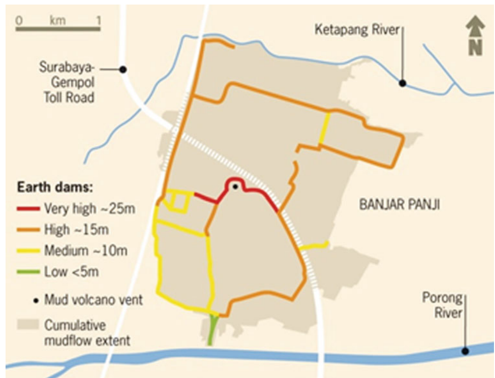
Fig. 21 Construction of permanent dykes (BPLS 2007)
