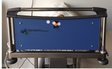
Fig. 2. NFC reader integrated into resident's bed
